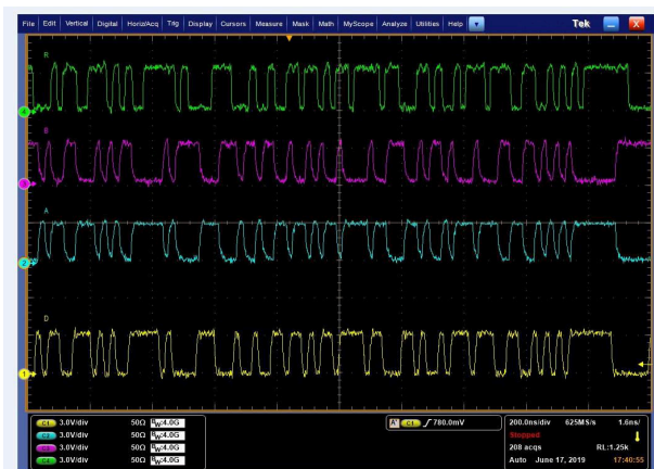
THVD2450 V_{CC} = 3.3\text{ V} R_L = 50\ \Omega Random (PRBS7) data at 50 Mbps
