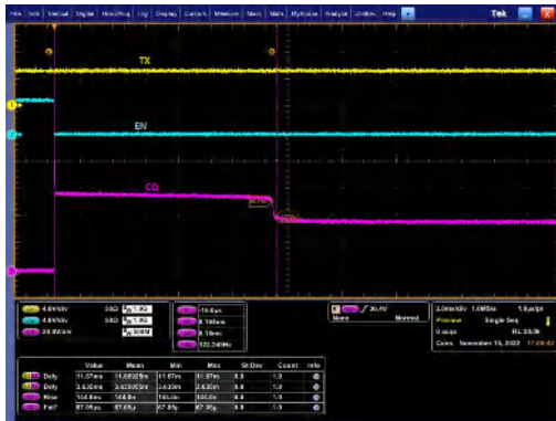
9-4. CQ in Current Fault Auto Recovery, Low Side Mode
