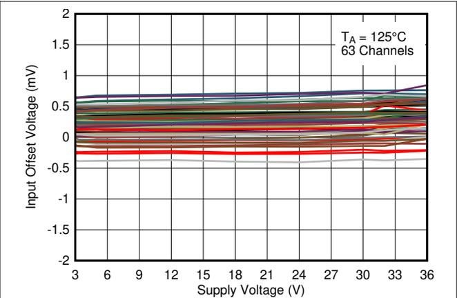
5-14. Input Offset Voltage vs. Supply Voltage at 125°C
