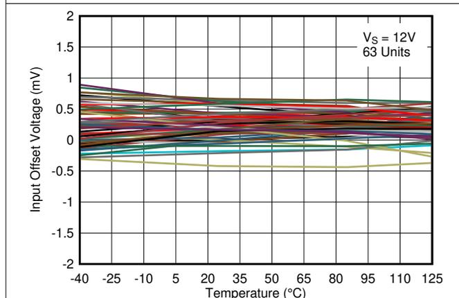
5-17. Input Offset Voltage vs. Temperature at 12V
