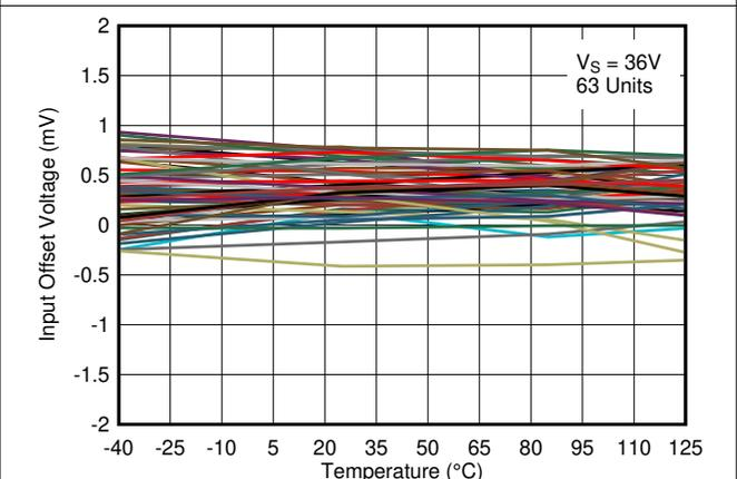
5-18. Input Offset Voltage vs. Temperature at 36V
