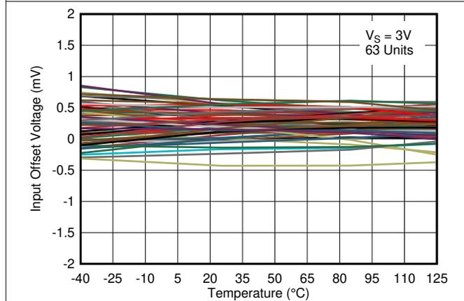
5-15. Input Offset Voltage vs. Temperature at 3V
