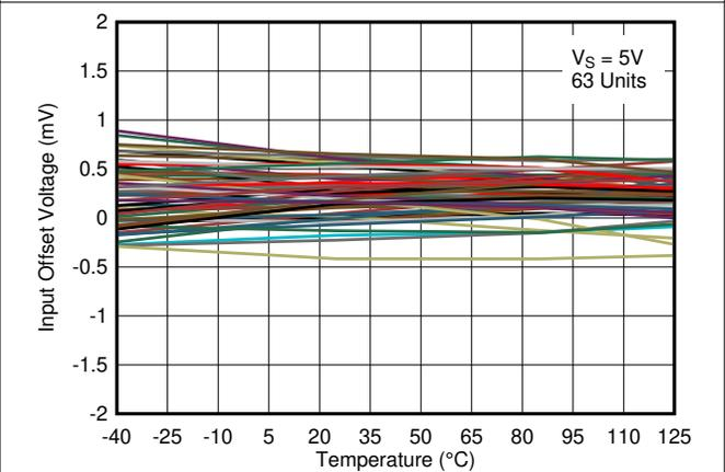
5-16. Input Offset Voltage vs. Temperature at 5V
