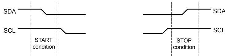
Figure 18-3. START and STOP Conditions
