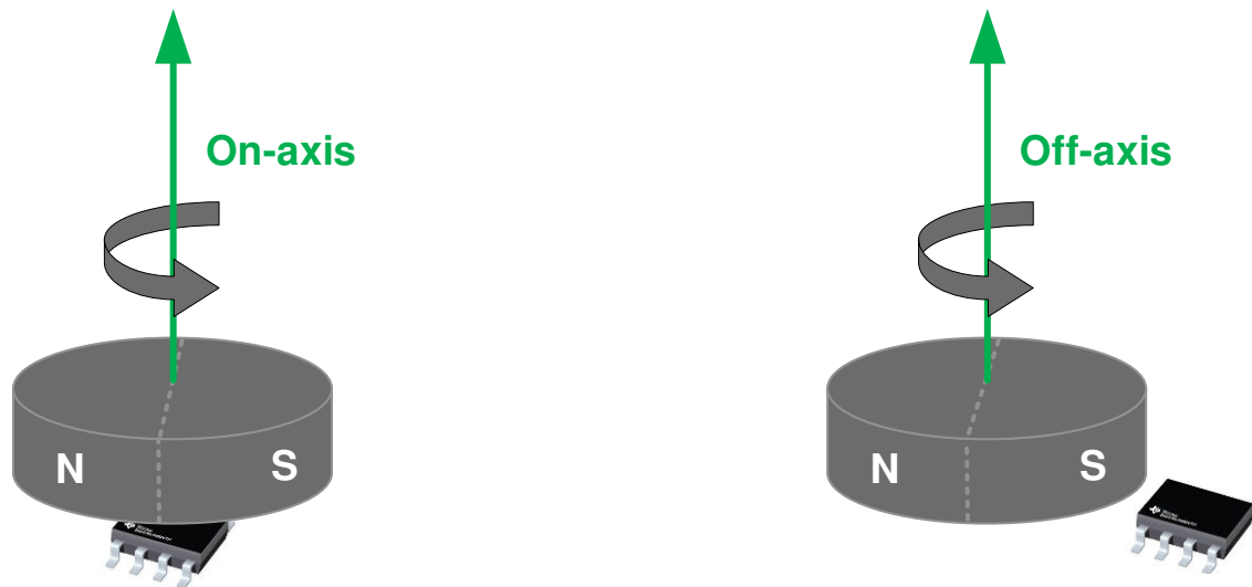
图 8-5. On-Axis vs. Off-Axis Angle Measurements
