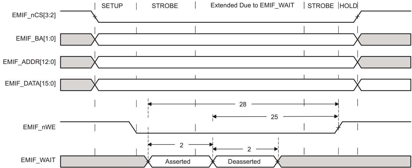
Figure 6-15. EMIFnWAIT Write Timing Requirements
