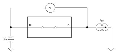
図 7-1. On-Resistance Measurement Setup
