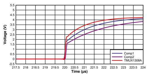
図 8-2. TMUX1308A vs. Competition Devices Drain Settling Times
