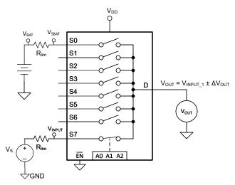
図 9-2. Channel S7 Selected, Channel S0 Experiencing a Short-to-Battery Condition
