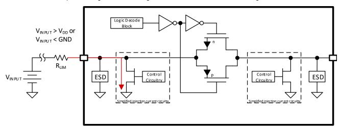
図 8-7. Over-Voltage Event with Series Resistor
