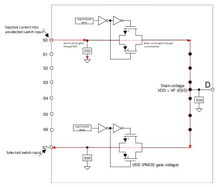
図 8-3. Simplified Diagram of Typical CMOS Switch and Associated Injected Current Path
