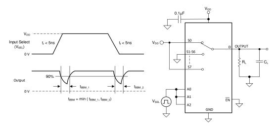
図 7-5. Break-Before-Make Delay Measurement Setup
