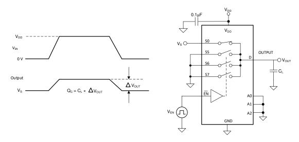
図 7-7. Charge-Injection Measurement Setup
