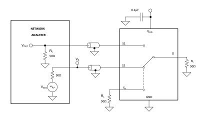
図 7-9. Channel-to-Channel Crosstalk Measurement Setup
