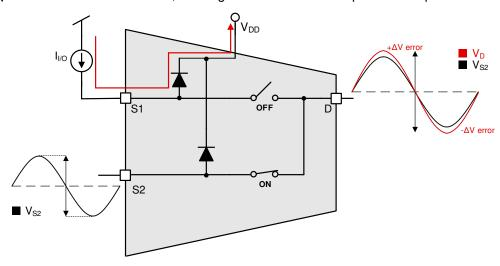
図 8-4. Injected Current Impact on RON
