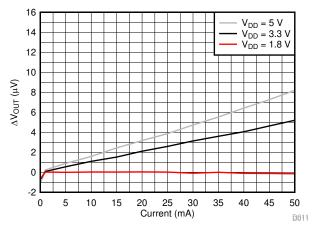
図 9-5. Injection Current vs. Maximum Output Voltage Shift
