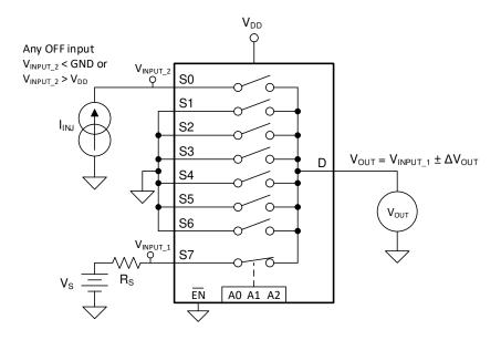
図 7-11. Injection Current Measurement Setup
