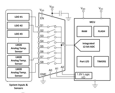
図 9-1. Multiplexing Signals to Integrated ADC
