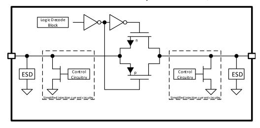
図 8-5. Simplified Diagram of Injection Current Control
