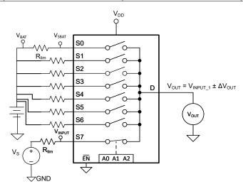
図 9-3. All Unselected Channels Experiencing a Short-to-Battery Condition
