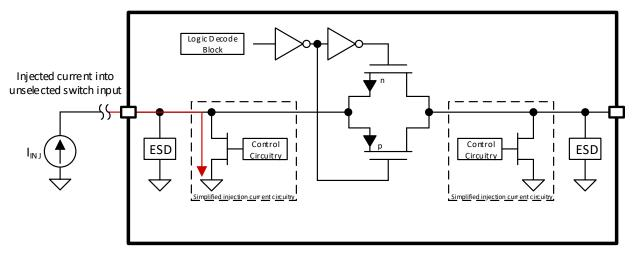
図 8-6. Injected Current at Input Pin
