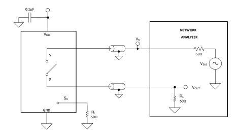
図 7-8. Off Isolation Measurement Setup
