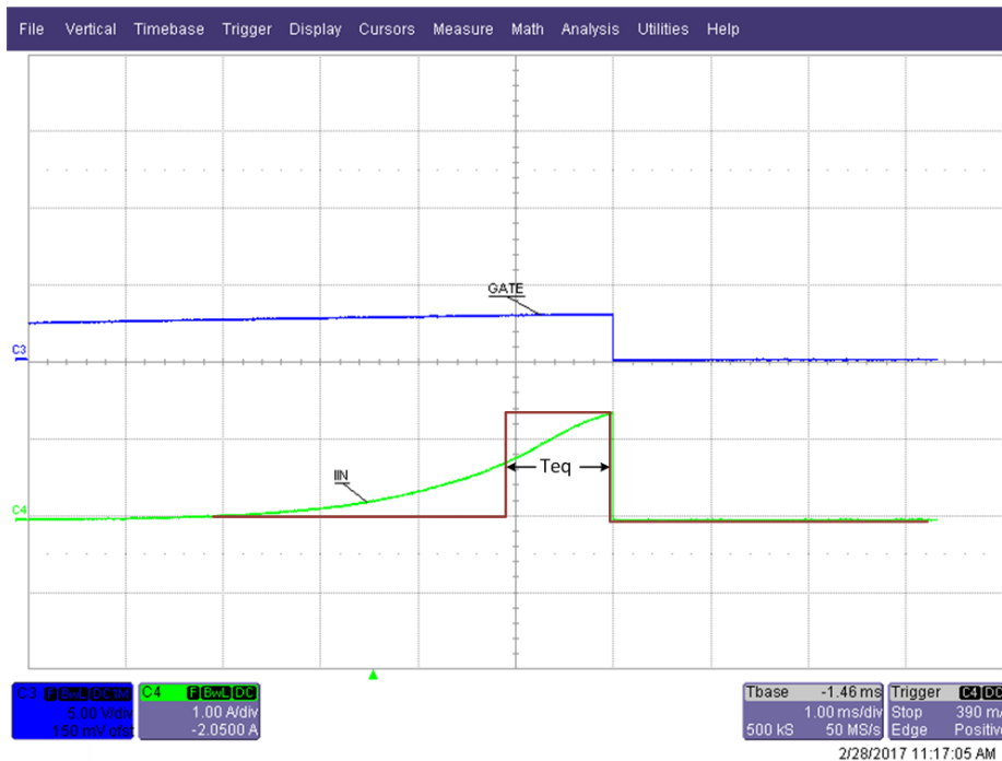
Figure 15. Teq During a Start Into a Short
