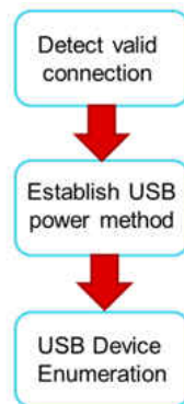
图 10-19. Flow of DFP-to-UFP Configuration
