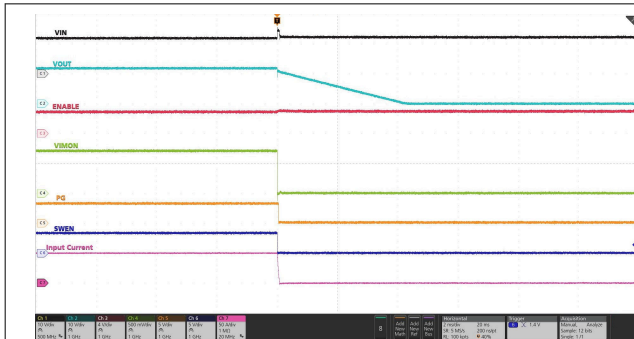
IN supply held steady at 12 V, EN pin held high, PMBus OPERATION OFF Command. C_{OUT} = 18\text{ mF} , C_{dVdt} = 33\text{ nF}
