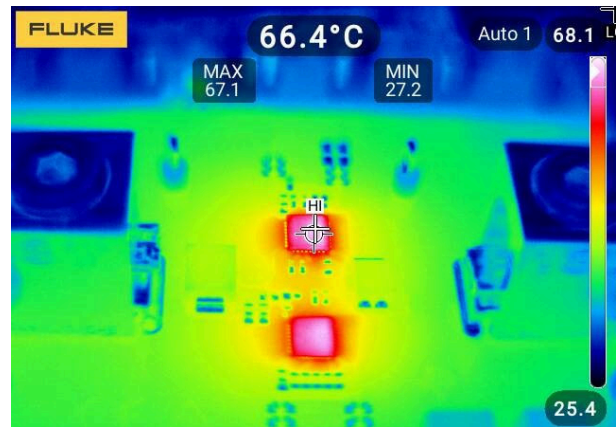
9-14. One (1) TPS25990 eFuse and one (1) TPS25985x eFuse in Parallel: Temperature Rise with 110-A DC Current at Room Temperature (No Air-Flow)
