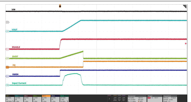
IN supply held steady at 12 V, EN pin toggled from low to high. C_{OUT} = 18\text{ mF} , C_{dVdt} = 33\text{ nF}
