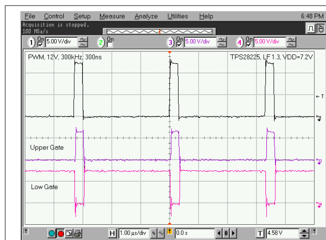
Fig 7-4. 12-V PWM Pulse at V_{DD} = 7.2\text{ V}
