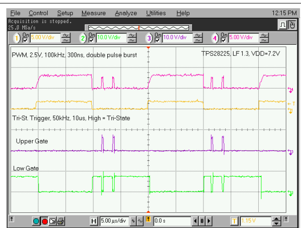
Figure 7-3. 2.5-V Amplitude PWM Pulse (TPS28225-Q1)
