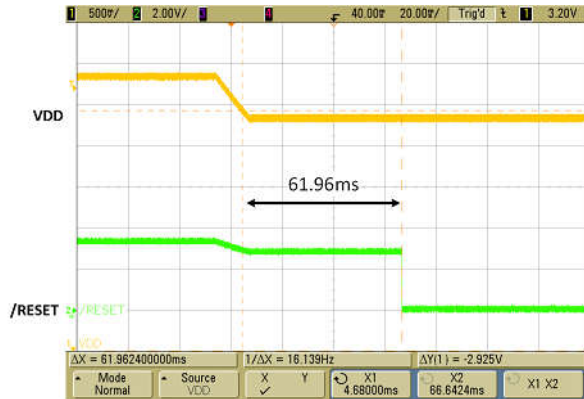
図 8-3. Sense Delay where CTS = 0.1 \mu F
