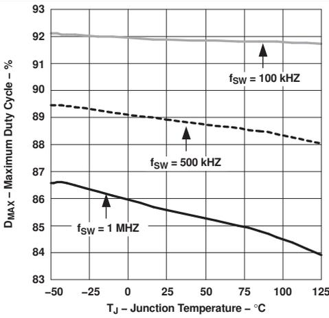
Figure 9. Maximum Duty Cycle vs Junction Temperature
