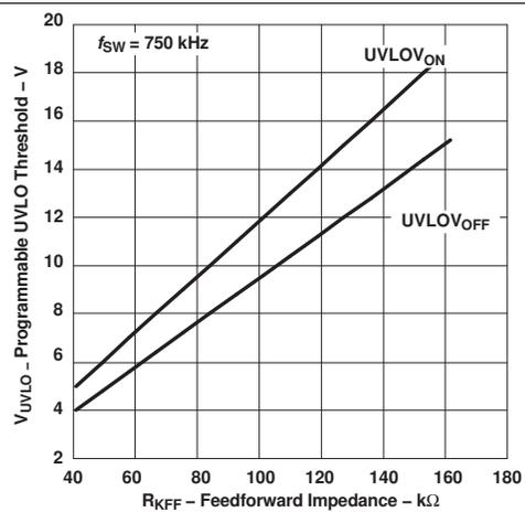
Figure 18. Undervoltage Lockout Threshold vs Feed-Forward Impedance
