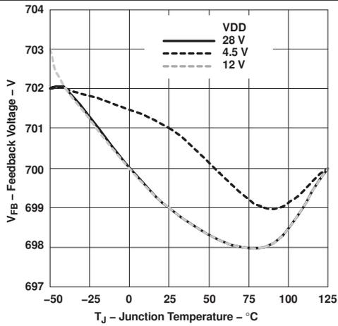
Figure 7. Feedback Regulation Voltage vs Junction Temperature
