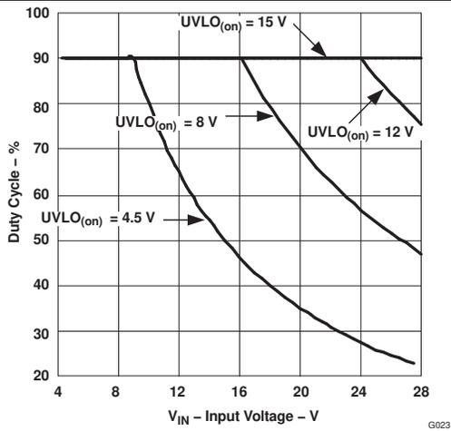
Figure 19. Typical Maximum Duty Cycle vs Input Voltage
