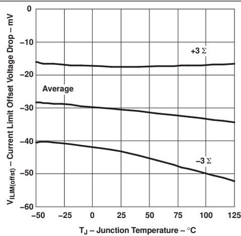
Figure 5. Current Limit Offset Voltage vs Junction Temperature
