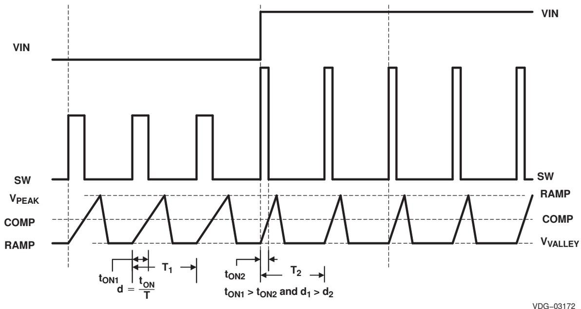
Figure 25. Voltage Feed-Forward and PWM Duty Cycle Waveforms
