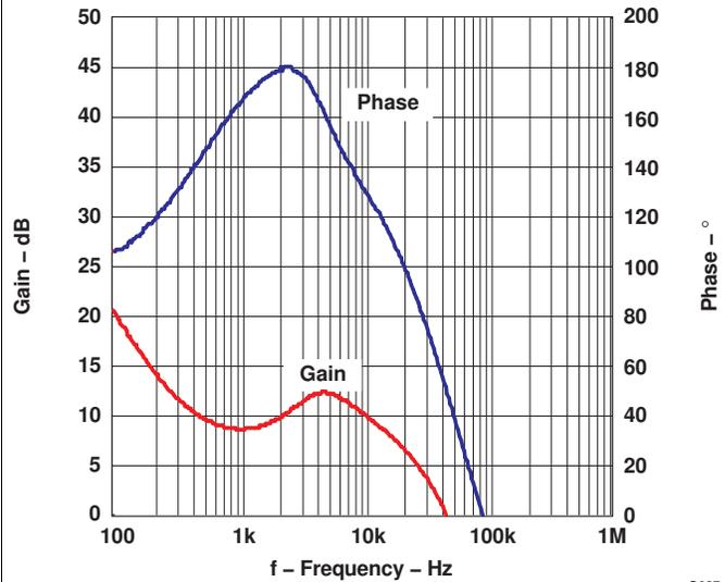
**Figure 33. Bode Plot Showing 57° Phase Margin
