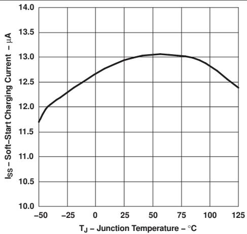
Figure 12. Soft-Start Charging Current vs Junction Temperature
