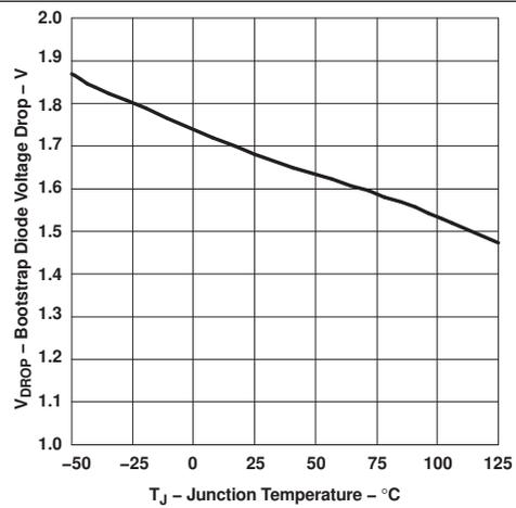
Figure 4. Bootstrap Diode Voltage vs Junction Temperature
