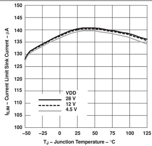
Figure 6. Current Limit Sink Current vs Junction Temperature
