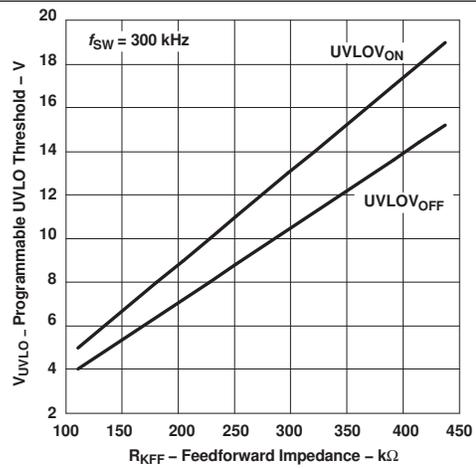
Figure 16. Undervoltage Lockout Threshold vs Feed-Forward Impedance
