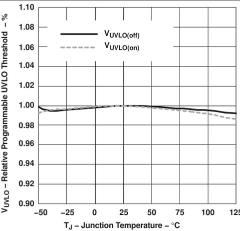
Figure 11. Programmable UVLO Threshold vs Junction Temperature
