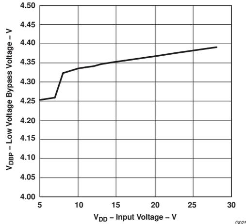
Figure 21. Input Voltage vs Low-Voltage Bypass Voltage
