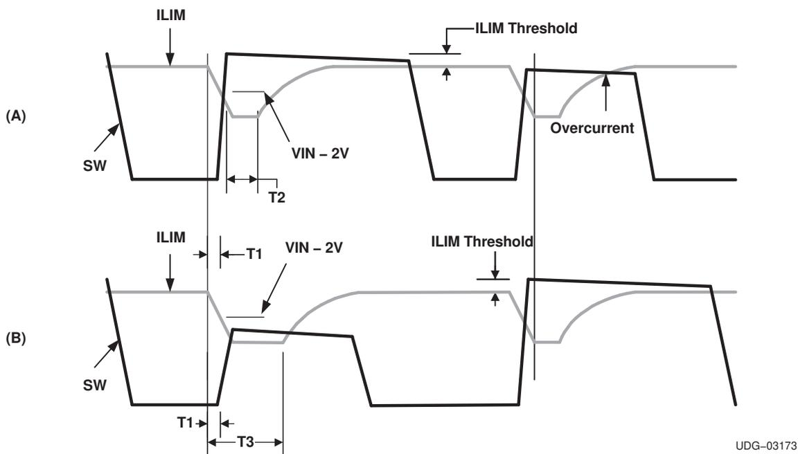
**Figure 26. Switching and Current-Limit Waveforms and Timing Relationship**
