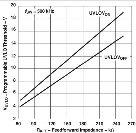
Figure 17. Undervoltage Lockout Threshold vs Feed-Forward Impedance
