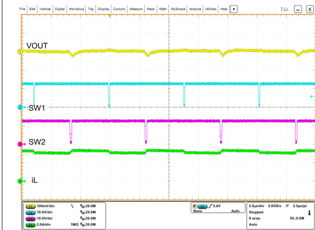
8-4. Switching Waveforms in V_{IN} = 12V , V_{OUT} = 12V , I_O = 3A , FPWM
