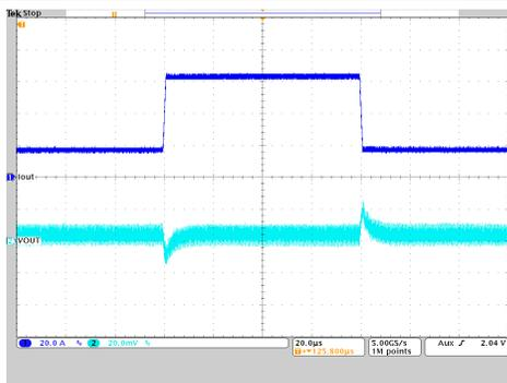
$V_{OUT} = 0.875V$  PWM; TPS62876  $T_A = 25^\circ C$
