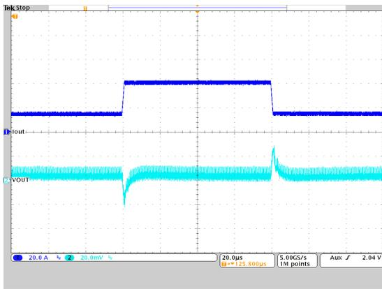
$V_{OUT} = 0.8V$       PWM; TPS62876       $T_A = 25^\circ C$
