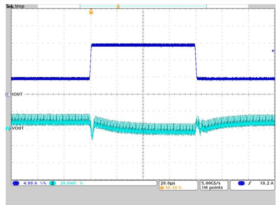
$V_{OUT} = 0.75V$       PWM, TPS62874 droop enabled       $T_A = 25^\circ C$
