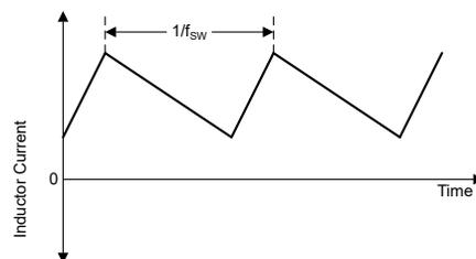
Figure 8-2. Continuous Conduction Mode (CCM) Current Waveform
