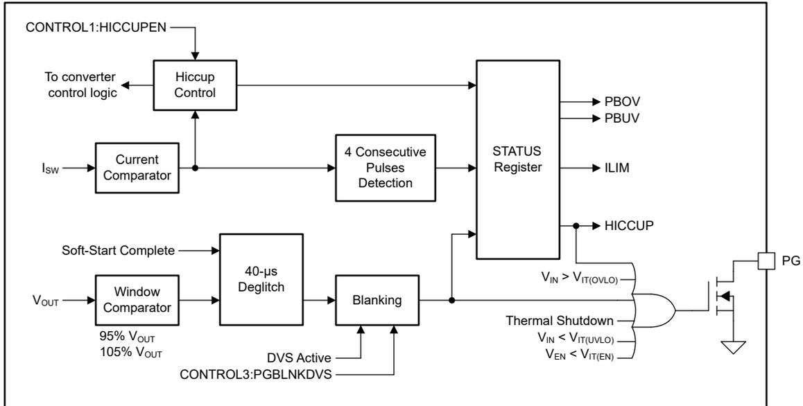
**図 8-14. Power-Good Functional Block Diagram (Standalone / Primary Device)**
