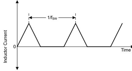
8-3. Discontinuous Conduction Mode (DCM) Waveform
