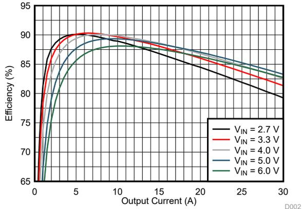
$V_{OUT} = 0.8V$       PWM       $T_A = 25^\circ C$
