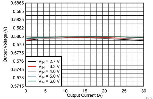
$V_{OUT} = 0.58V$  PWM; droop disabled  $T_A = 25^\circ C$
