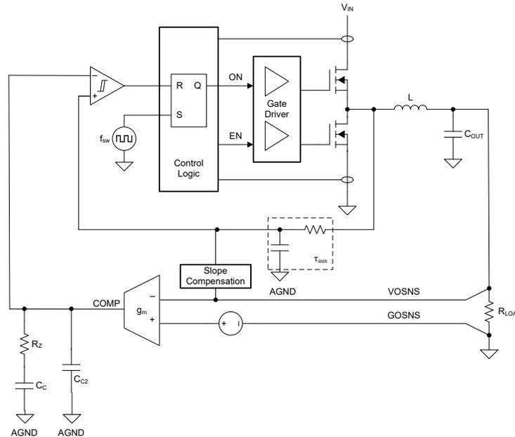
Figure 8-1. Fixed-Frequency DCS-Control Topology (Simplified)
