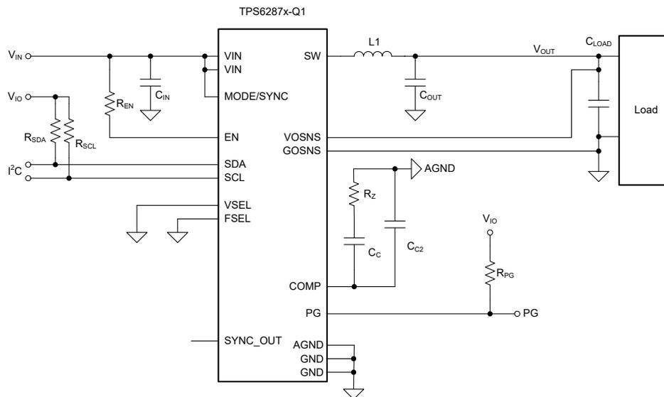
図 10-1. Typical Application Schematic
