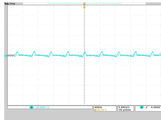
$V_{OUT} = 0.75V$       PWM       $T_A = 25^\circ C$
