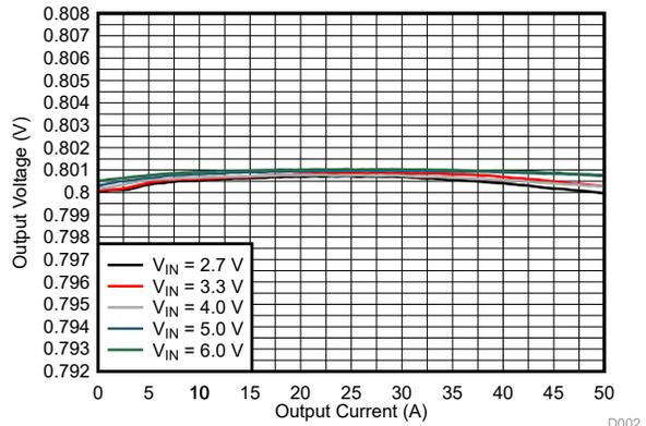
$V_{OUT} = 0.8V$  PWM  $T_A = 25^\circ C$
