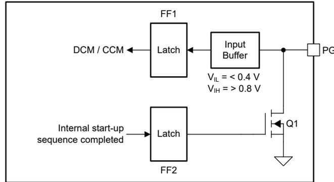
❑ 8-15. Power-Good Functional Block Diagram (Secondary Device)
