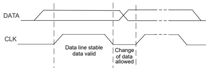
図 8-18. Bit Transfer on the Serial Interface
