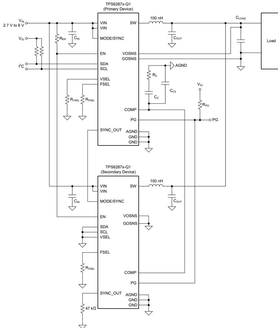
☒ 8-16. Two TPS6287x-Q1 Devices in a Stacked Configuration
