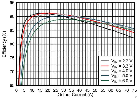
$V_{OUT} = 0.875V$  PWM  $T_A = 25^\circ C$
