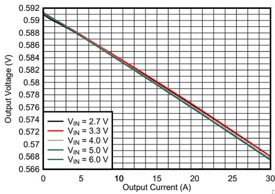
$V_{OUT} = 0.58V$  PWM; TPS62877 droop enabled  $T_A = 25^\circ C$
