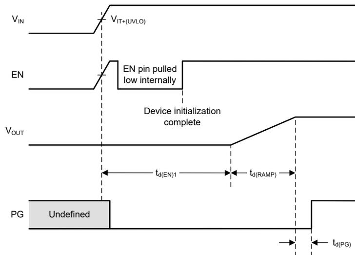
☒ 8-7. Start-Up Timing When EN is Pulled Up to V<sub>IN</sub>
