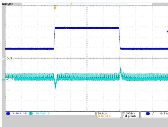
$V_{OUT} = 0.75V$       PWM, TPS62874 droop disabled       $T_A = 25^\circ C$
