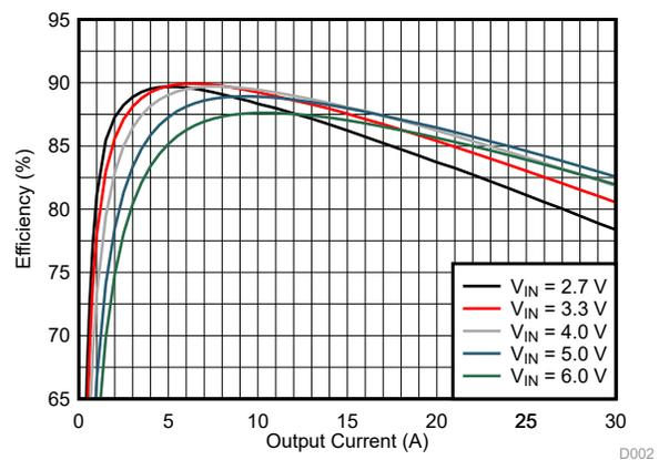
$V_{OUT} = 0.75V$  PWM  $T_A = 25^\circ C$
