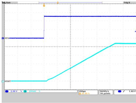
$V_{OUT} = 0.875V$  PWM  $T_A = 25^\circ C$
