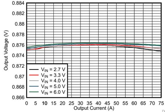
$V_{OUT} = 0.875V$  PWM  $T_A = 25^\circ C$
