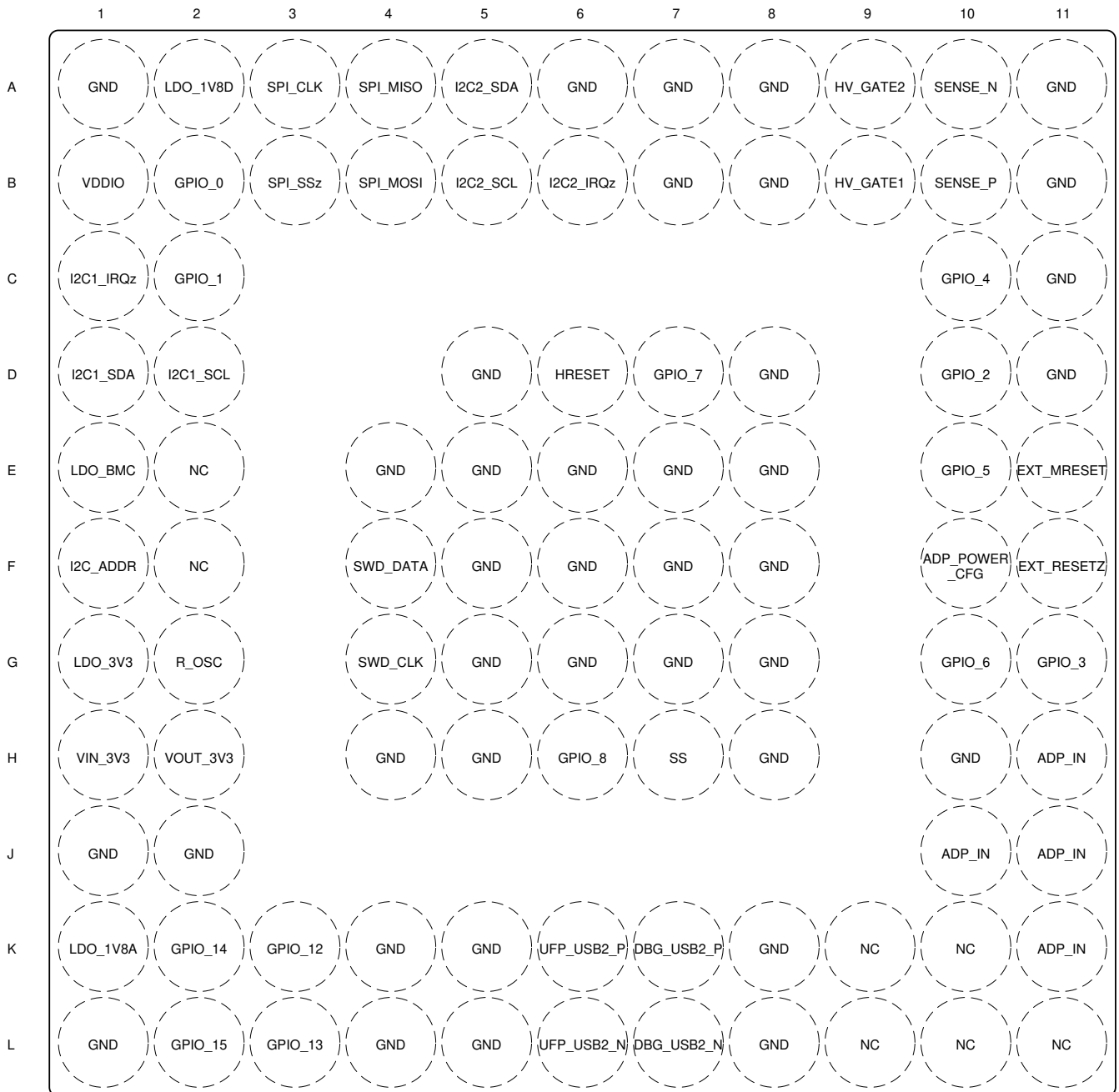
5-1. ZBH Package 96-Pin NFBGA Top View
