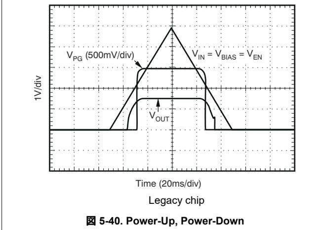
Figure 5-40. Power-Up, Power-Down
