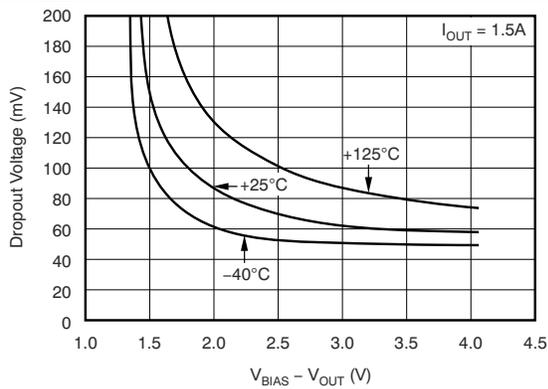
5-11.  $V_{IN}$  Dropout Voltage vs  $(V_{BIAS} - V_{OUT})$  and Temperature ( $T_A$ )
