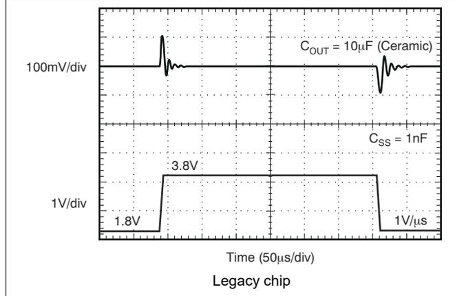
Figure 5-34. V<sub>IN</sub> Line Transient
