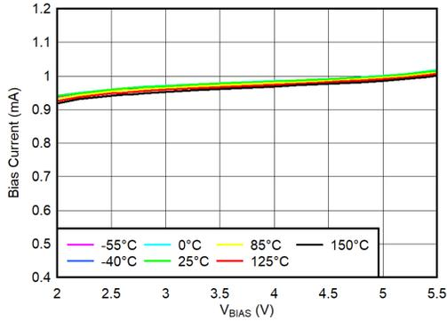
**Figure 5-25. BIAS Pin Current vs V<sub>BIAS</sub> and Temperature (T<sub>J</sub>)**
