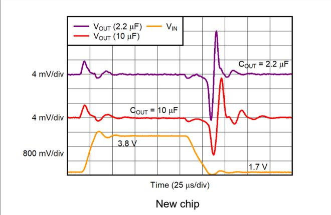
Figure 5-35. V<sub>IN</sub> Line Transient
