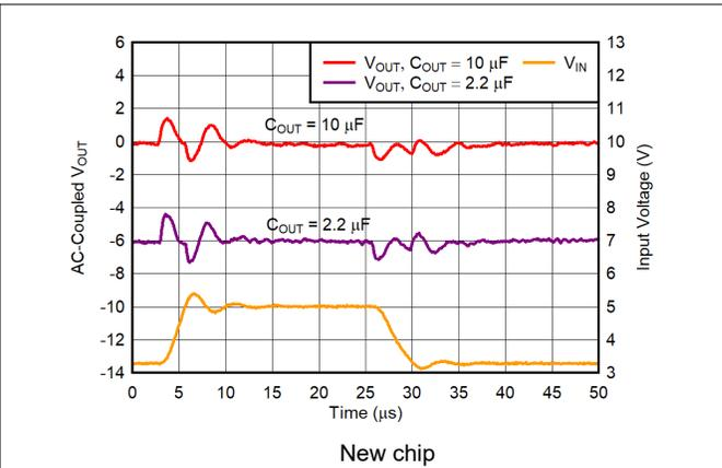
Figure 5-33. V<sub>BIAS</sub> Line Transient
