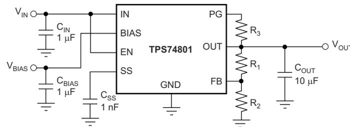
$$V_{\text{OUT}} = 0.8 \times \left( 1 + \frac{R_1}{R_2} \right)$$
