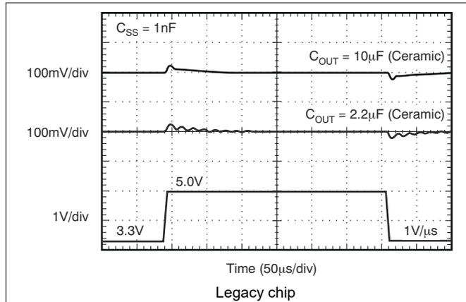
Figure 5-32. V<sub>BIAS</sub> Line Transient
