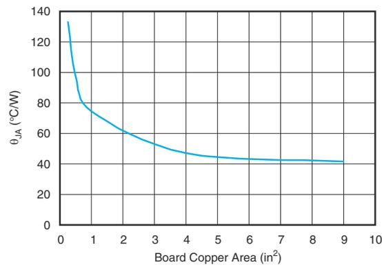
$R_{\theta JA}$  value at board size of 9 in<sup>2</sup> (that is, 3-in × 3-in) is a JEDEC standard.
