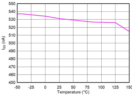
**Figure 5-27. Soft-Start Charging Current (I<sub>SS</sub>) vs Temperature (T<sub>J</sub>)**
