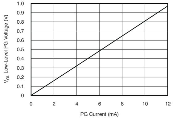
**Figure 5-28. Low-Level PG Voltage vs Current**
