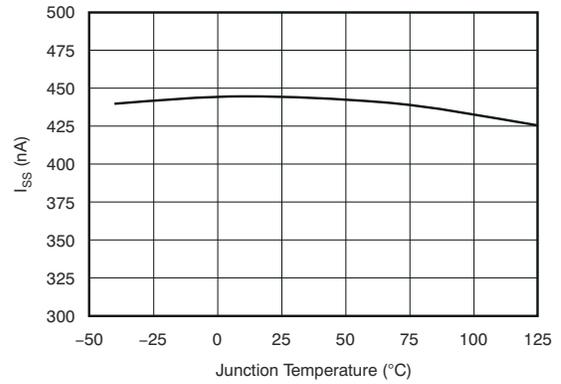
**Figure 5-26. Soft-Start Charging Current (I<sub>SS</sub>) vs Temperature (T<sub>J</sub>)**
