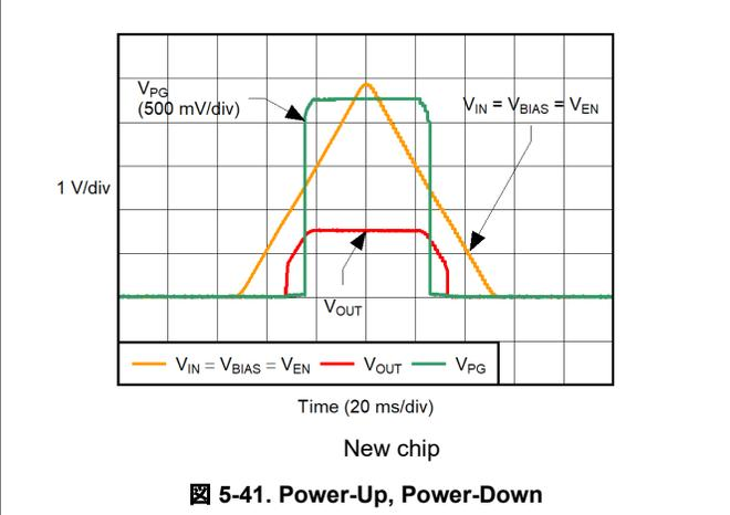
Figure 5-41. Power-Up, Power-Down
