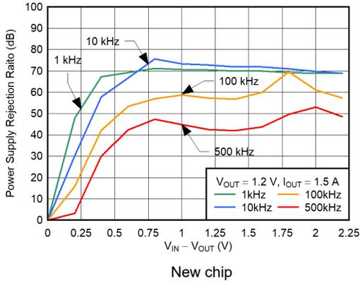
5-19.  $V_{IN}$  PSRR vs  $(V_{IN} - V_{OUT})$
