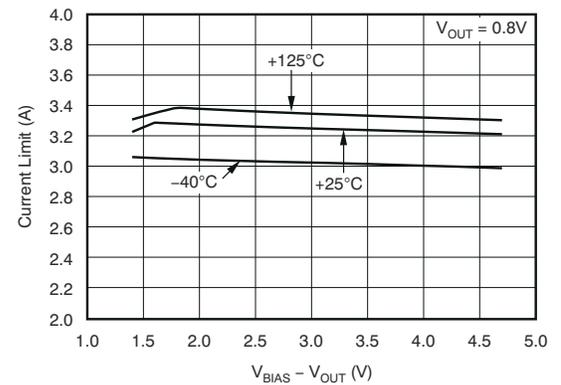
**Figure 5-30. Current Limit vs (V<sub>BIAS</sub> - V<sub>OUT</sub>)**
