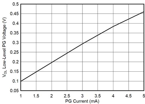
**Figure 5-29. Low-Level PG Voltage vs Current**
