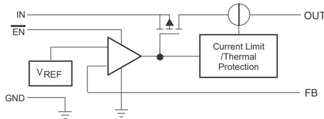
图 6-1. TPS76901 Functional Block Diagram (Legacy Chip)
