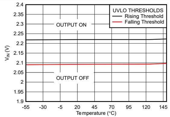
5-18. TPS76933 UVLO Threshold vs Free-Air Temperature (New Chip)
