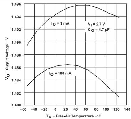
図 5-6. TPS76915 Output Voltage vs Free-Air Temperature (Legacy Chip)
