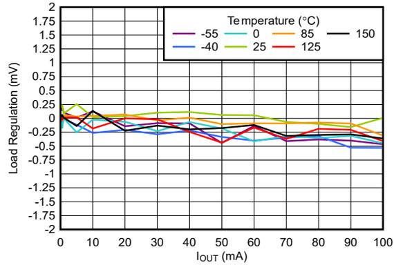
Figure 5-11. TPS76933 Load Regulation vs Free-Air Temperature (New Chip)
