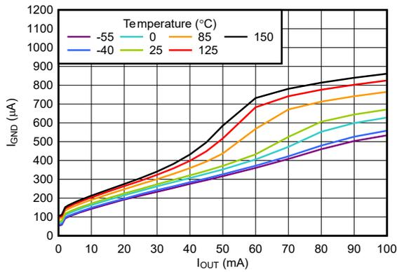
5-15. TPS76933 Ground Current vs Output Current (New Chip)
