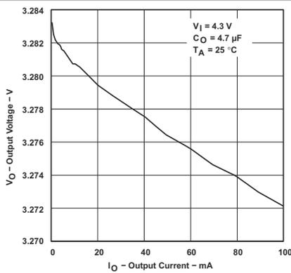
図 5-3. TPS76933 Output Voltage vs Output Current (Legacy Chip)
