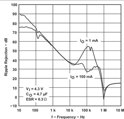
図 5-30. TPS76933 Ripple Rejection vs Frequency (Legacy Chip)
