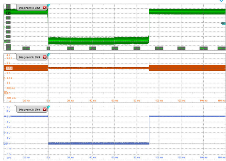
Ch2: Output voltage (1 V/div); Ch3: LED current (500 mA/div); Ch4: FLT voltage (1 V/div); Time: 20 ms/div
