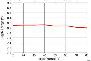
Figure 14. VCC vs Input Voltage
