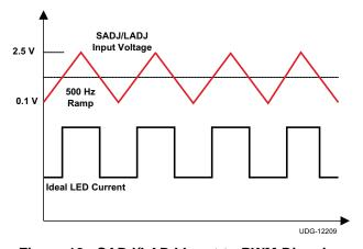
Figure 18. SADJ/LADJ Input to PWM Dimming
