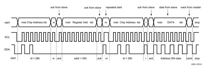
Figure 24. I<sup>2</sup>C Read Cycle
