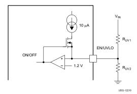
Figure 19. Input UVLO Circuit
