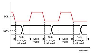
Figure 20. I<sup>2</sup>C Signals: Data Validity
