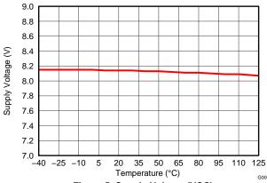
Figure 5. Supply Voltage (VCC) vs Junction Temperature
