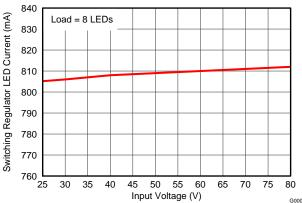
Figure 9. Switching Regulator LED Current vs Input Voltage
