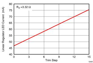
Figure 12. Linear Regulator LED Current vs I<sup>2</sup>C Trim Step
