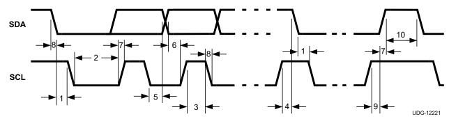
Figure 25. I<sup>2</sup>C Timing Diagram
