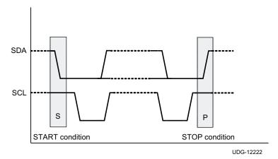
Figure 21. I<sup>2</sup>C Start and Stop Conditions
