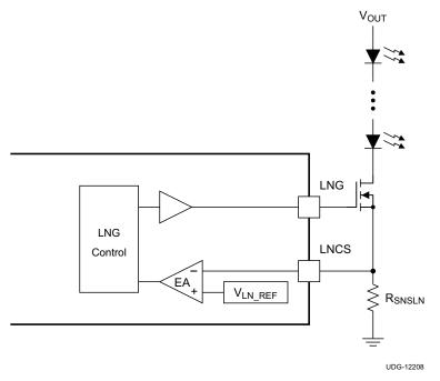
Figure 17. Linear Regulator Control
