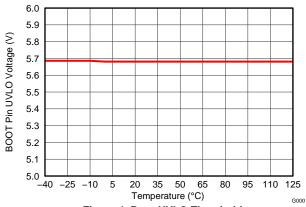
Figure 4. Boot UVLO Threshold vs Junction Temperature
