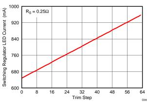
Figure 11. Switching Regulator LED Current vs I<sup>2</sup>C Trim Step
