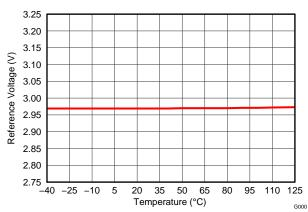
Figure 6. Voltage Reference vs Junction Temperature
