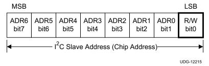
Figure 22. I<sup>2</sup>C Chip Address
