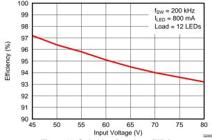
Figure 13. Switching Regulator Efficiency vs Input Voltage
