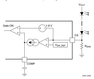
Figure 15. Current Control Circuitry
