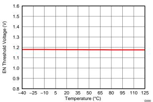
Figure 3. Enable Threshold Voltage vs Junction Temperature
