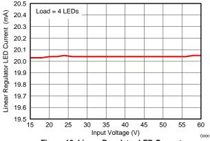
Figure 10. Linear Regulator LED Current vs Input Voltage
