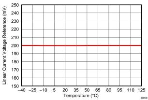
Figure 7. Linear Current Voltage Regulation vs Junction Temperature
