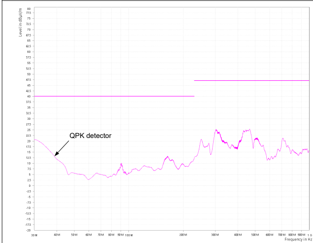
9-10. CISPR 32 Class B Radiated Emissions: Horizontal Polarization
