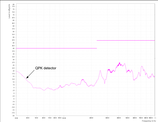
9-11. CISPR 32 Class B Radiated Emissions: Vertical Polarization
