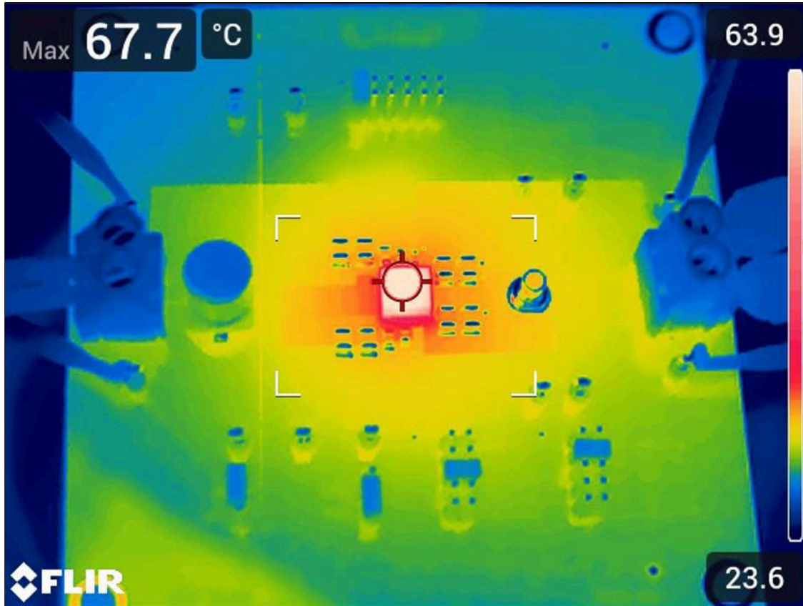
8-17. Thermal Image at 25^\circ\text{C} Ambient
