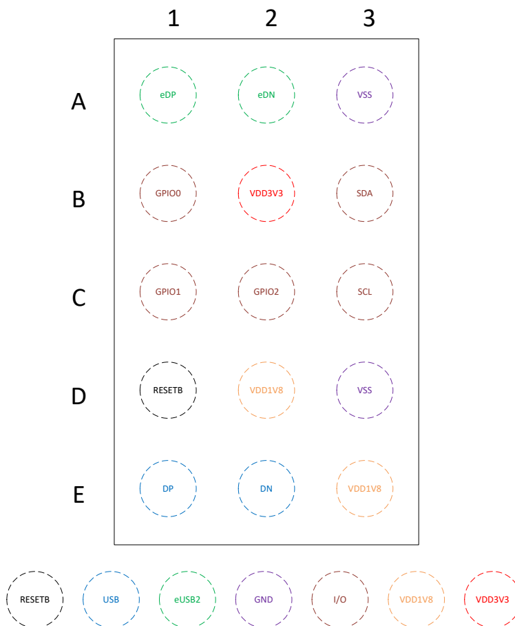
図 5-1. TUSB2E11 YCG Package, 15-Pin DSBGA (Top View)
