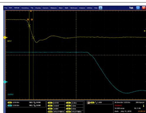
図 8-13. PWM Input (yellow) and Driver Output (blue) Falling Edge
