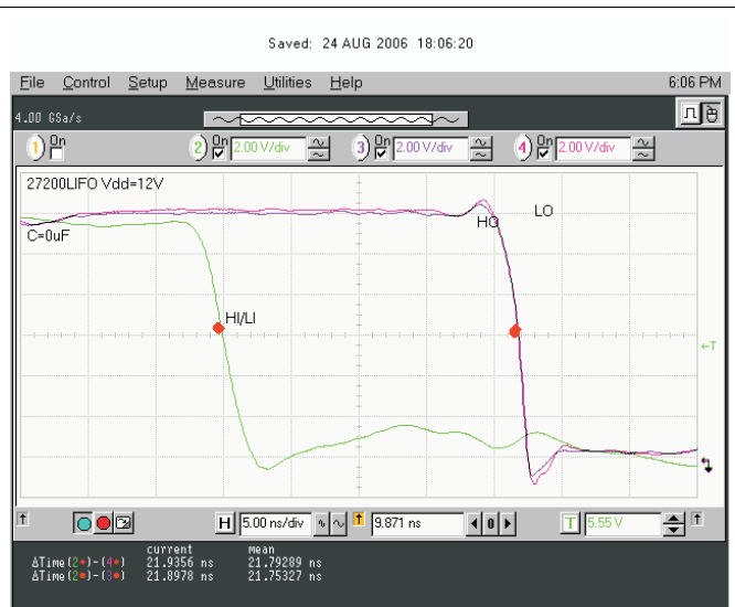
Figure 31. V_{LO} and V_{HO} Falling Edge Delay Matching
