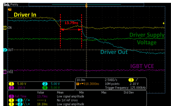
8-3. UCC27624-Q1 Used to Drive IGBT in the Boost Converter
