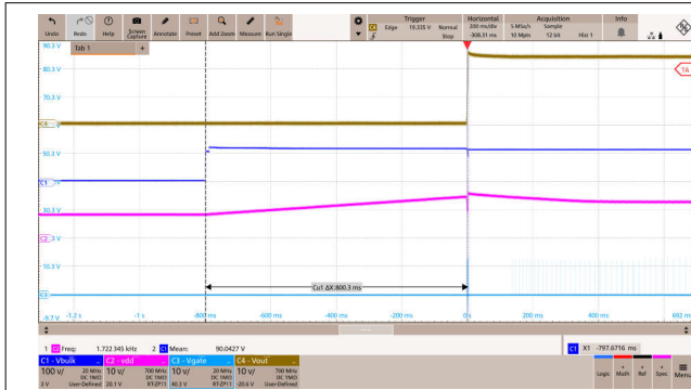
図 8-4. Start-Up Waveforms at 85Vac and No Load
