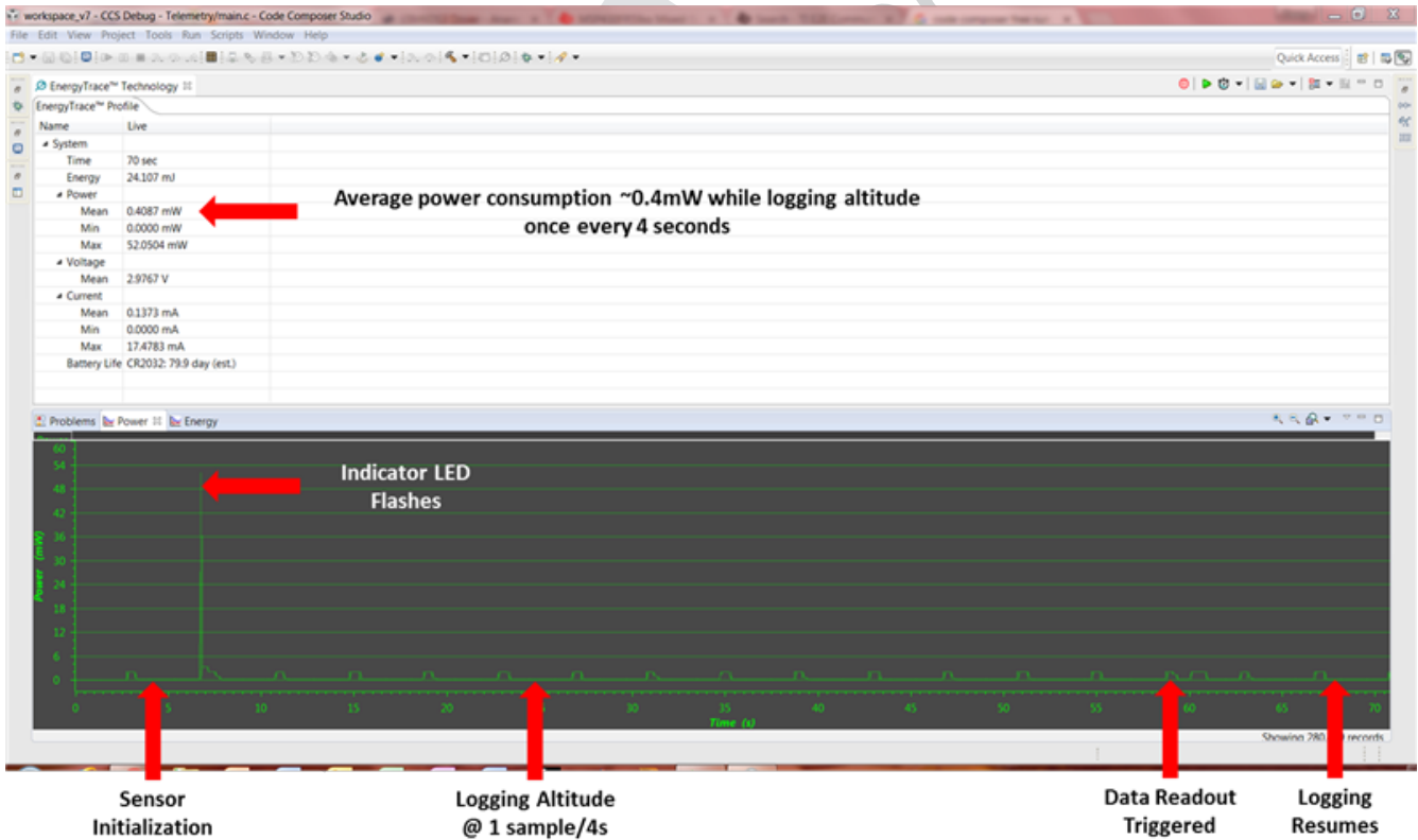
Figure 2. MSP430 EnergyTrace Software with a Two-sample-per-second Measurement Frequency
