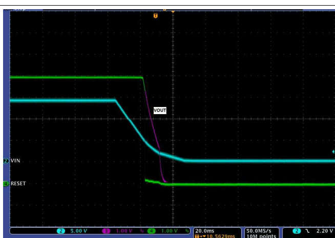
Figure 24. TPS7B6750-Q1 Power-Down Waveform
