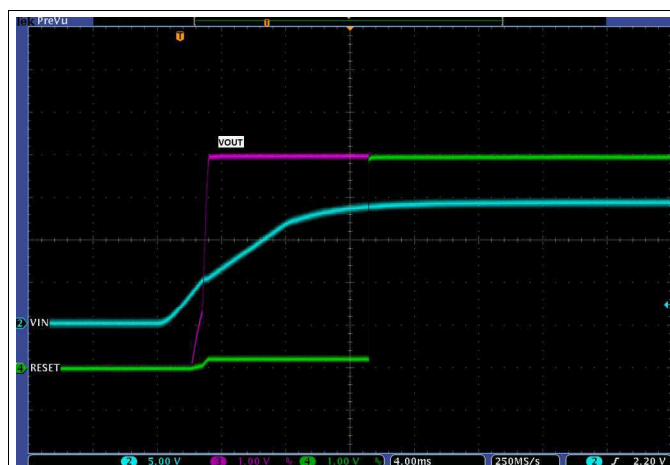
Figure 23. TPS7B6750-Q1 Power-Up Waveform
