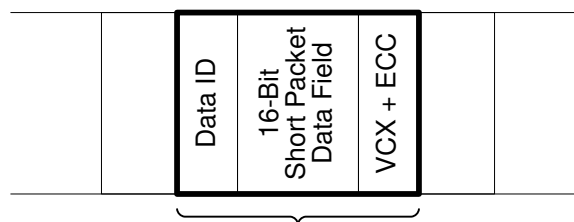
32-bit SHORT PACKET (SH) Data Type (DT) = 0x00 – 0x0F
