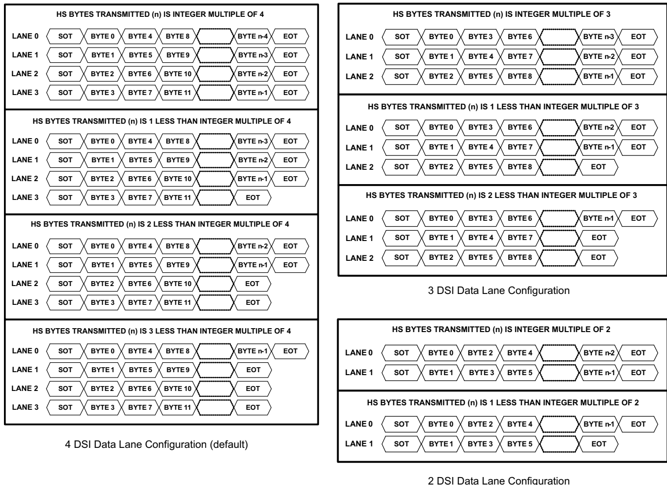
Figure 13. SN65DSI83-Q1 DSI Lane Merging Illustration
