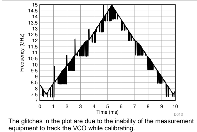
Figure 11. VCO Ramping 7.5-GHz to 15-GHz Triangle Wave With VCO Calibration
