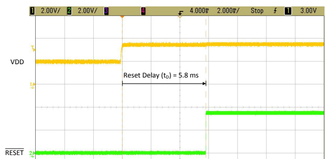
⊗ 54. TPS3840EVM \overline{\text{RESET}} Time Delay ( t_D ) with 0.01- \mu\text{F} Capacitor
