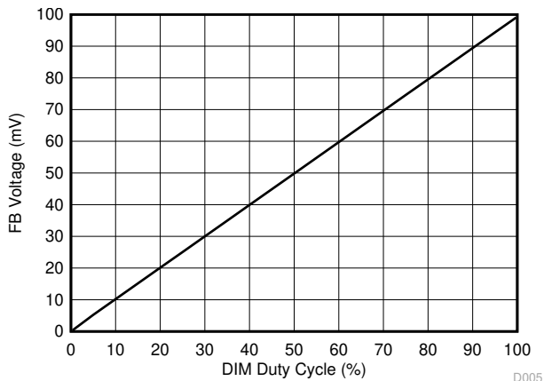
6-5. DIM Duty Cycle vs FB Voltage in Analog Dimming (for TPS92200D2)
