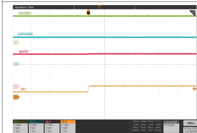
9-15. ORing V_{IN2} to V_{IN1} Switch Over
