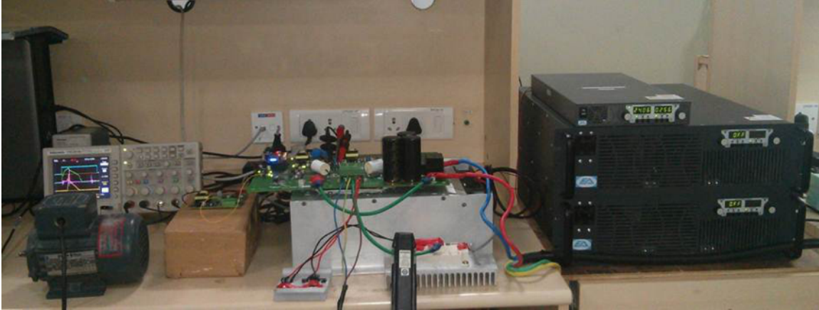
☒ 101. Setup for Short Circuit Test — Fault Under Load
