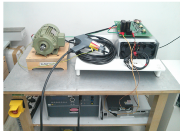
図 115. EUT/AUX Equipment Isolated From Reference Plane by 10 cm
