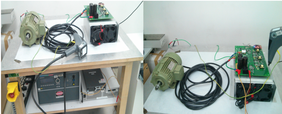
図 113. EUT/AUX Equipment on Insulated Sheet
