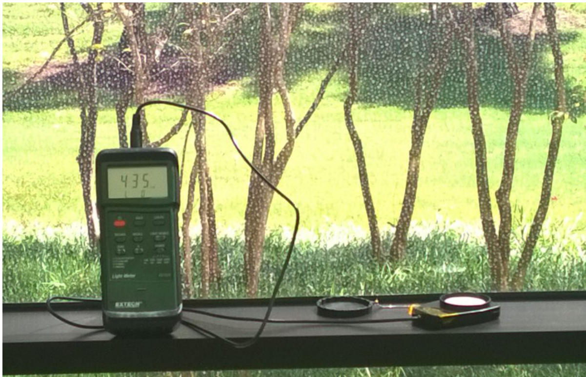
図 18. Light Meter Measuring Light Level in a Sunny Window
