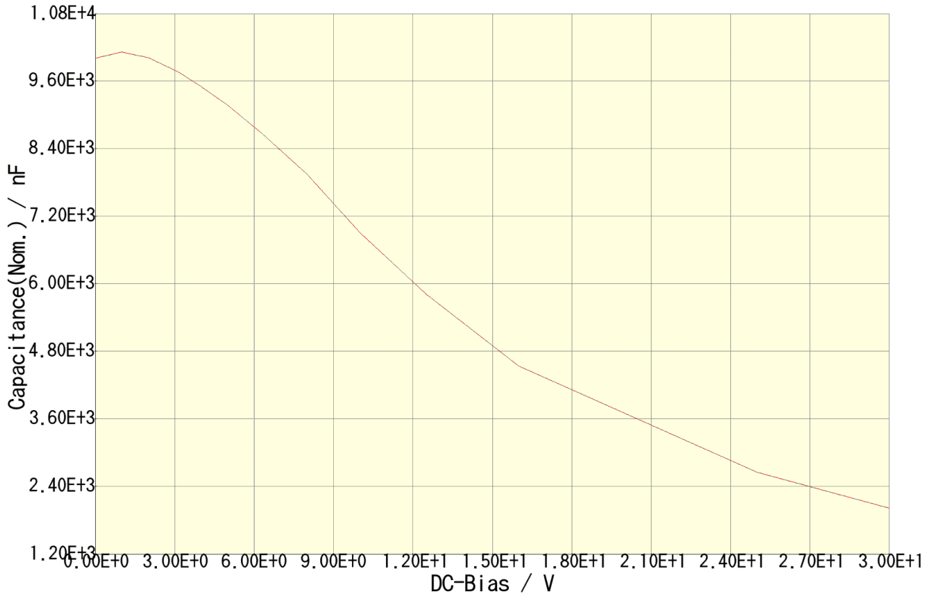
図 7. Variation of Capacitance With Applied DC Bias for C3216X7R1V106K160AC
