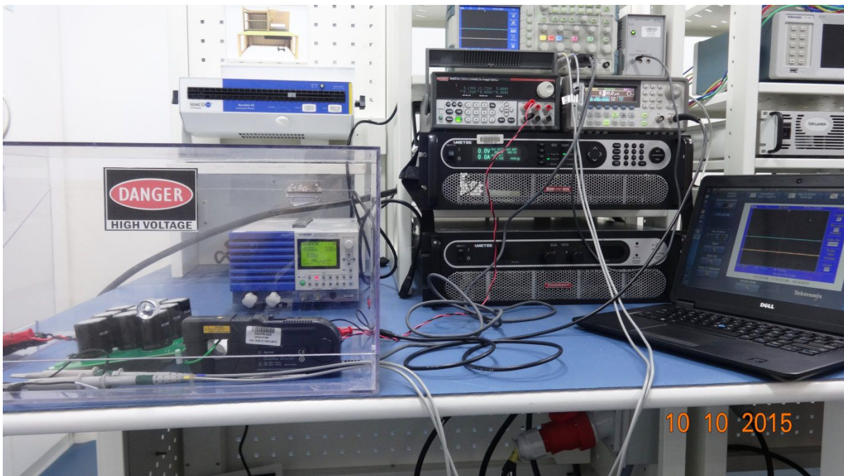
図 75. Miller Clamp and Desaturation Detection Test Setup
