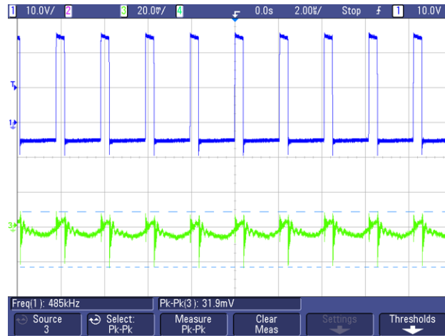
☒ 94. SW Node Waveform and Output Ripple for V_{OUT} = -5\text{ V} , I_{OUT} = -1\text{ A}
