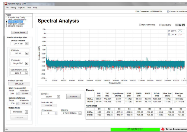
☒ 26. ADC AC Performance With a Gain of 10 at 2 kHz Using 18-Bit ADS8910B
