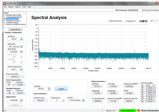
Figure 16. ADC Performance at 2-kHz Input With Gain of 1
