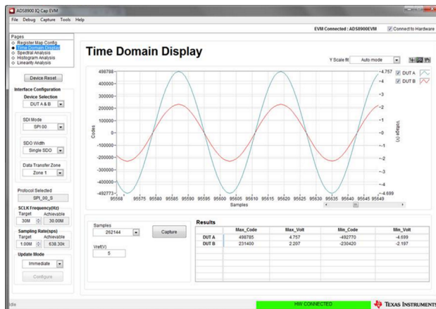
☒ 24. Time Domain Display of I and Q Signals at 20 kHz (One Channel is Given Half of the Gain Compared to the Other Channel)
