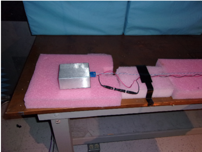
Figure 37. Slave Node Setup for RE per CISPR 25 ALSE
