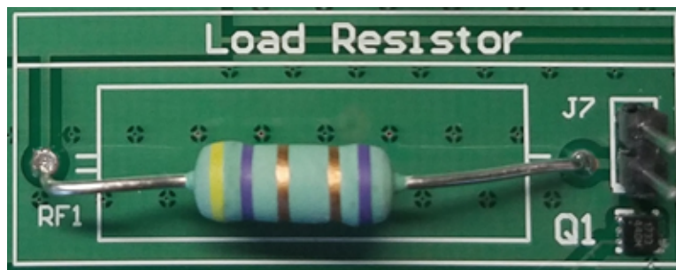
Figure 18. Dummy Load Resistor Circuitry on PCB
