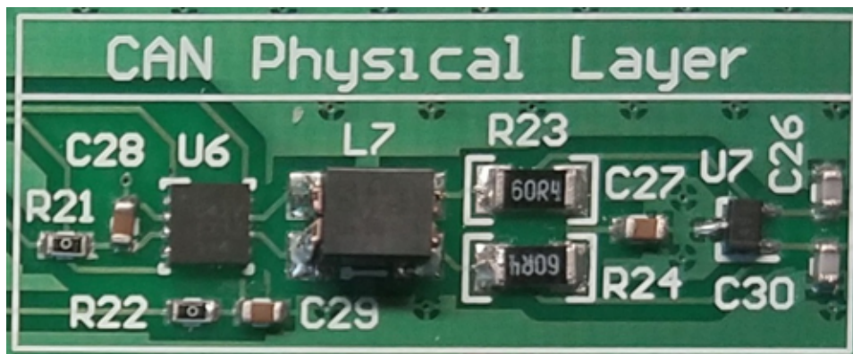
Figure 14. CAN Physical Layer Circuitry on PCB
