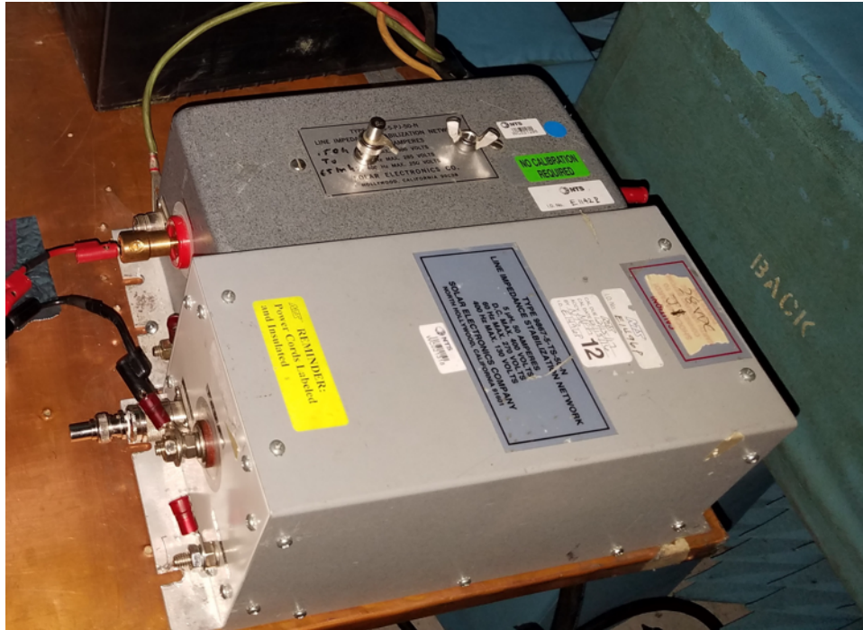
Figure 50. Two Artificial Networks With Measuring Ports for Conducted Emissions Testing
