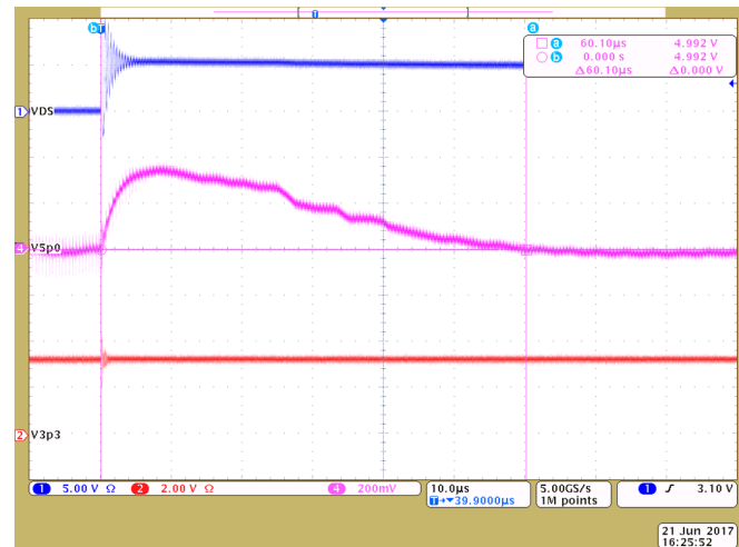
Figure 48. Buck Converter Load Step Decrease Recovery Time
