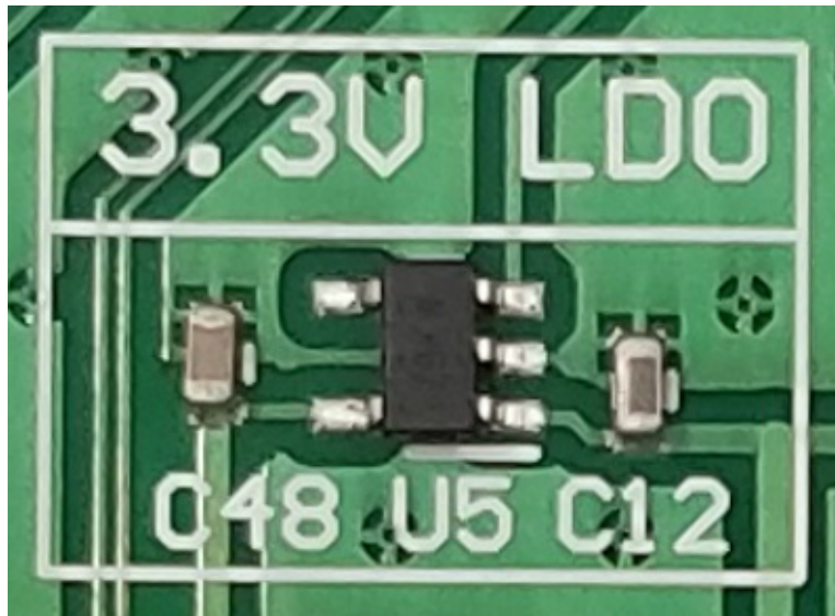
Figure 17. TLV71333P-Q1 LDO Circuitry on PCB
