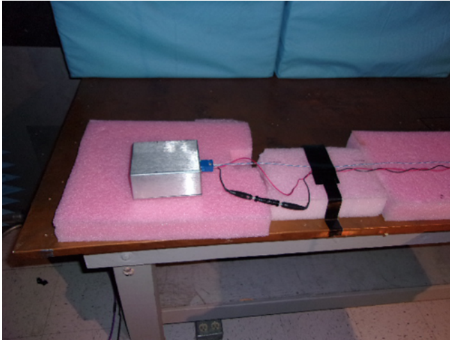
☒ 51. Slave Node Setup for Radiated Emissions
