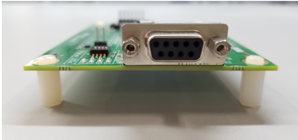
図 21. External Connector for Power and CAN on PCB
