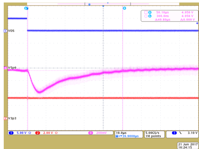
Figure 46. Buck Converter Load Step Increase Recovery Time
