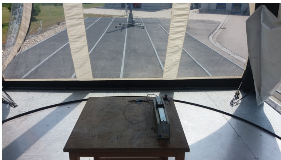
図 28. Radiated Emission 10-m Test Setup
