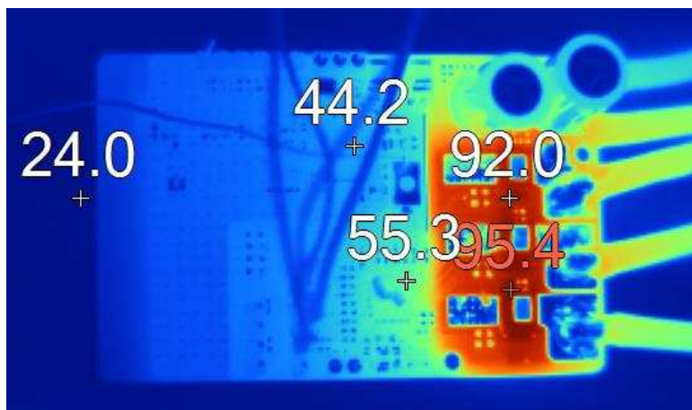
図 27. Thermal Image at 18-V DC Input, 25.6-A RMS Winding Current, 100% Duty Cycle
