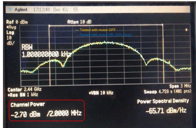
☒ 39. Measured TX Channel Power Measurement at 2440 MHz, 0-dBm Level With Motor ON and OFF
