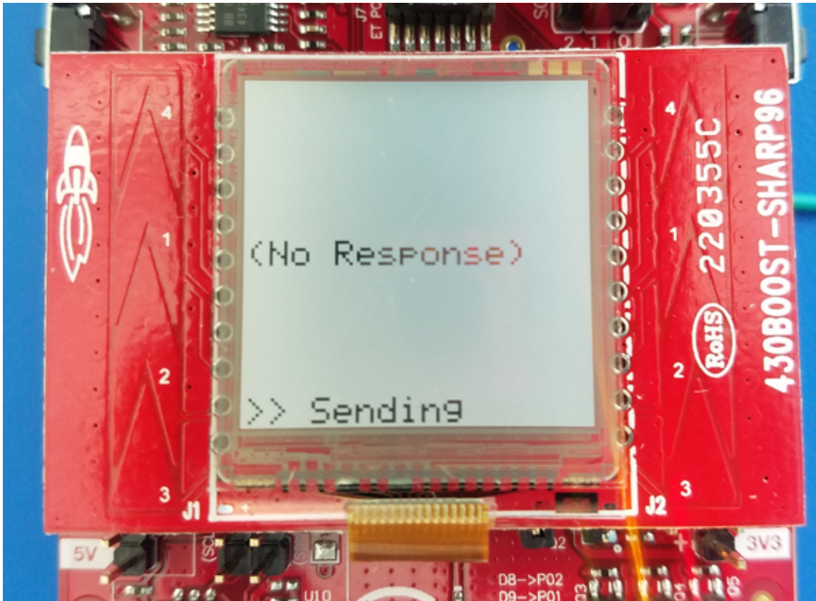
図 46. Sharp® LCD Indicates Sending Audio to IBM Watson® Servers in Progress
