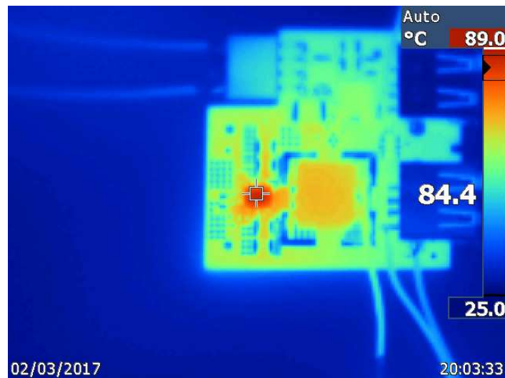
Figure 4. Thermal Image at Full Load
