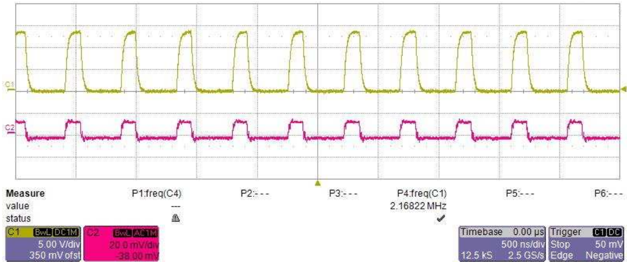
Figure 19. LM73605-Q1 Switch Node and Output Voltage Ripple, 13.5-V Input at Full Load
