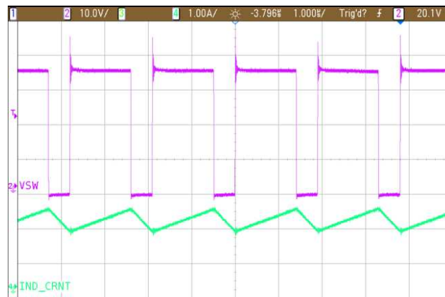
Figure 16. Buck Stage Switching Waveform
