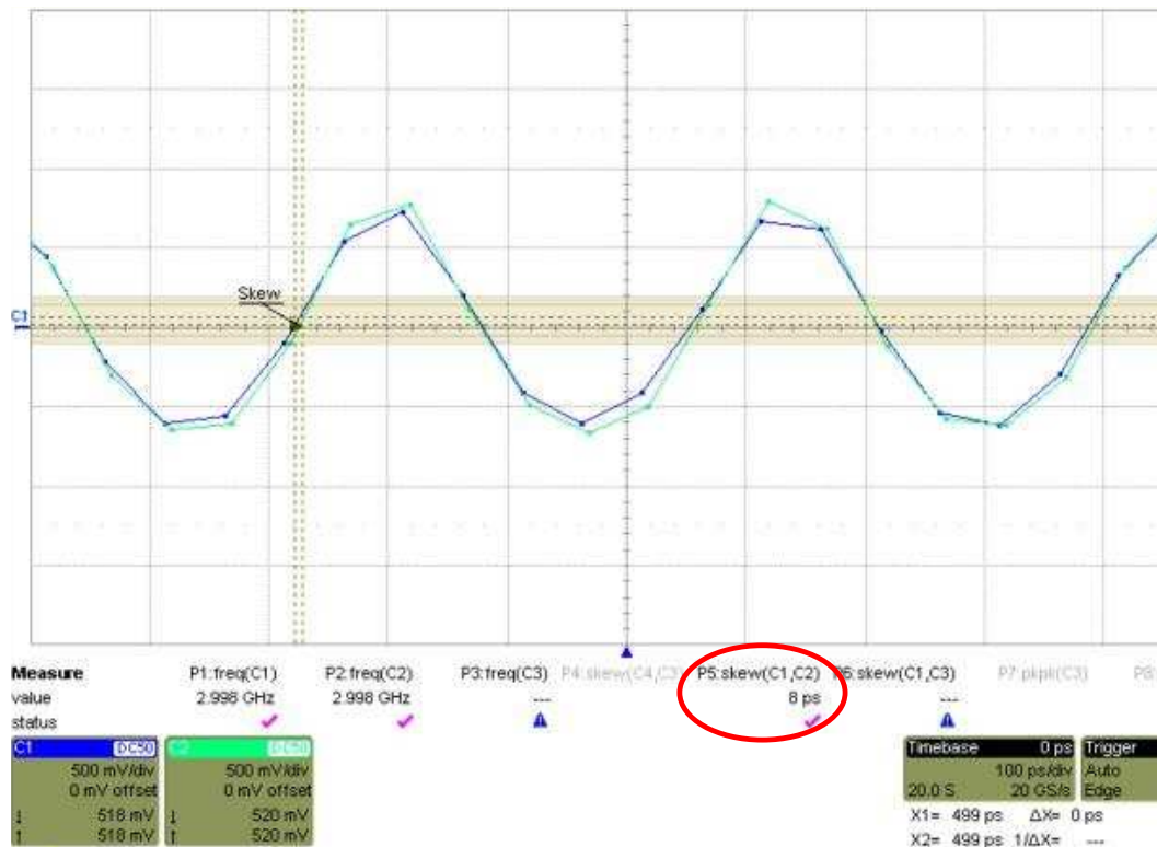
図 13. Board-to-Board Clock Measured Skew
