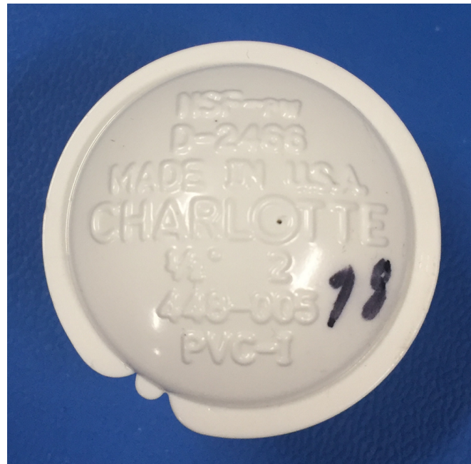
Figure 5. Cap With Hole for Test Leak Apparatus
